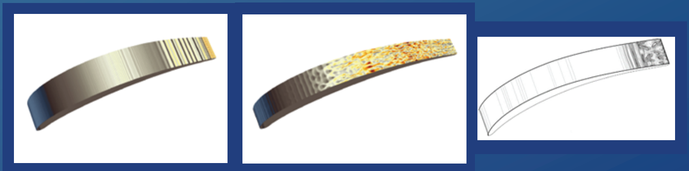
Figure (3): The instantaneous velocity on the blade surface to visualise transition. (a) clean inlet, (b) with inlet disturbance and (c) velocity normal to surface (clean inlet)
